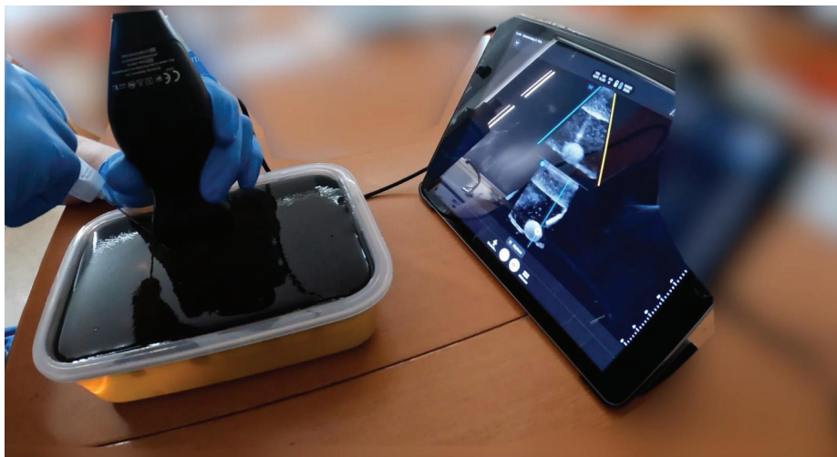
Figure 3. Intervention setting. The tablet screen displays the biplane mode. The top half of the screen shows the short-axis (out-of-plane) view, while the bottom half depicts the long-axis view. The operator uses the biplane mode to perform an ultrasound-guided biopsy in the presented gel phantom.
